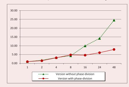
Figure 1. Comparison of acceleration in parallel calculation depending on the number of processors with different number of agents
