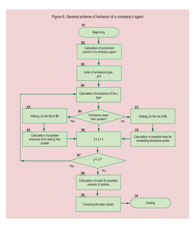
**B2**. In this block, using the production function, we calculate the volume of production of a company agent at the current number of agent workers and the level of technological development.
