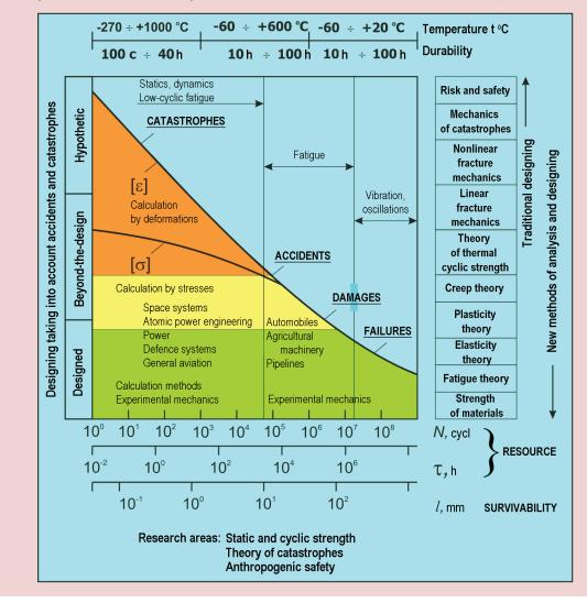
approach, the durability of structures ranging from 100 seconds to hundreds and thousands of hours at temperatures *t* from  $-270^{\circ}$ C to 1000 degrees°C, at the numbers of cycles *N* from 10<sup>0</sup> to  $10^9 - 10^{10}$ , temporary resource  $\tau$  from  $10^{-2}$  to  $10^6$  hours, at the linear dimensions of defects *l* from  $10^{-2}$  to  $10^3$  mm.
